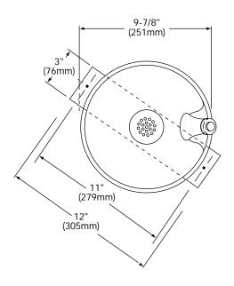
NOTE: ROUGH-IN DIMENSIONS MAY VARY 1/2" (13mm) PLUS OR MINUS. BUBBLER CAN BE MOUNTED ON RIGHT OR LEFT AS DESIRED.
