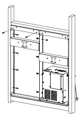
Remove left hand mounting frame, replace with new open frame (included)
