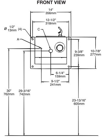
Note: A service supply stop must be installed at the fountain inlet line.
