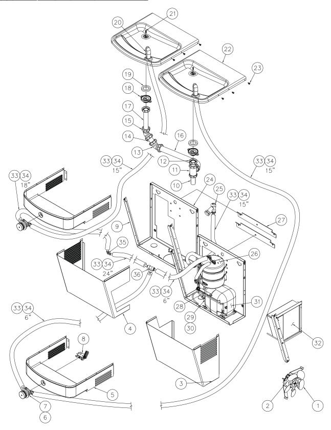
Standard A112408B-FG-VR 14 Gage Stainless Steel Enhanced Vandal Resistance Refrigerated Bi-Level AquaAccess shown.
