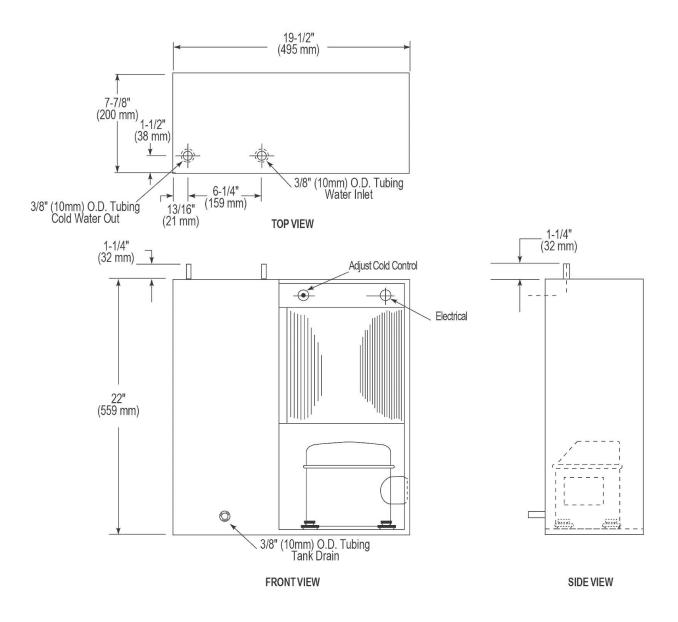
NOTE: It is important to insure proper ventilation. Allow a minimum clearance of 6" (152 mm) in front and 3"(76 mm) in the rear of the unit. If unit is to be installed in an enclosure, allow the following clearances around unit: 1"(25 mm) each side, 3"(76 mm) in the rear, 3"(76 mm) above.
