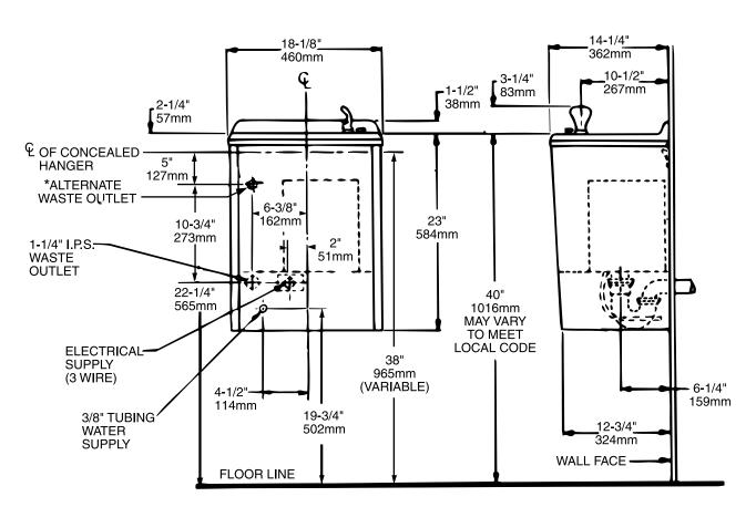
NOTE: Optional holes may be added to back panel to secure bottom of cooler to wall. Minimum wall clearance for air flow is 4 inches (102mm) on either side.
