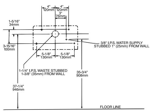
Note: A service supply stop (not included) must be installed at the fountain inlet line. 1-1/4" trap provided.
