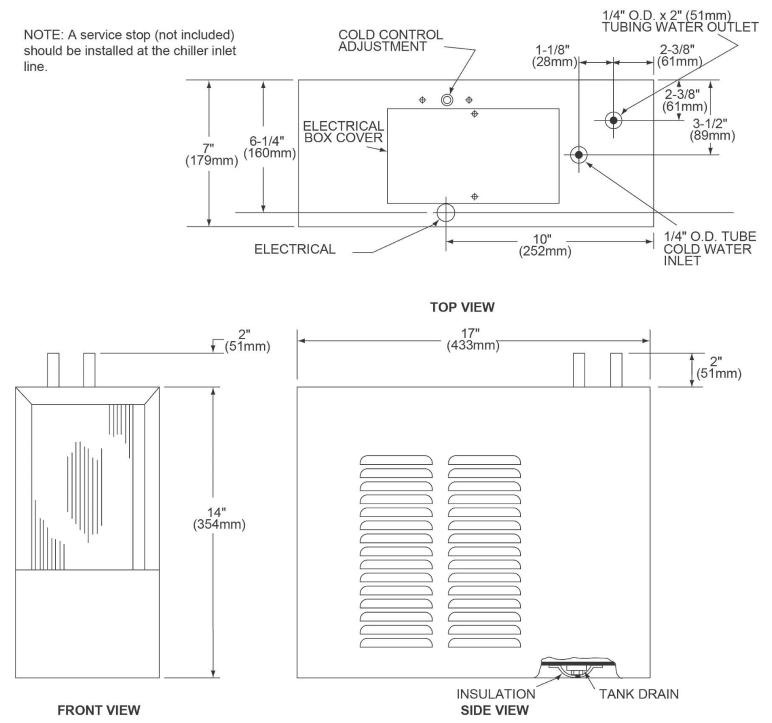
NOTE: It is important to insure proper ventilation. If this remote chiller is physically placed against barrier or in enclosure of any kind, 4" (102mm) air space must be allowed on all sides.
