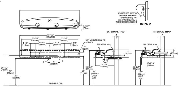
B = WATER OUTLET 1-1/2" O.D. DRAIN STUB OUT FROM WALL 1" (25mm)
