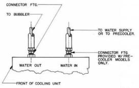
SIDE VIEW OF COOLING UNIT CONNECTIONS
