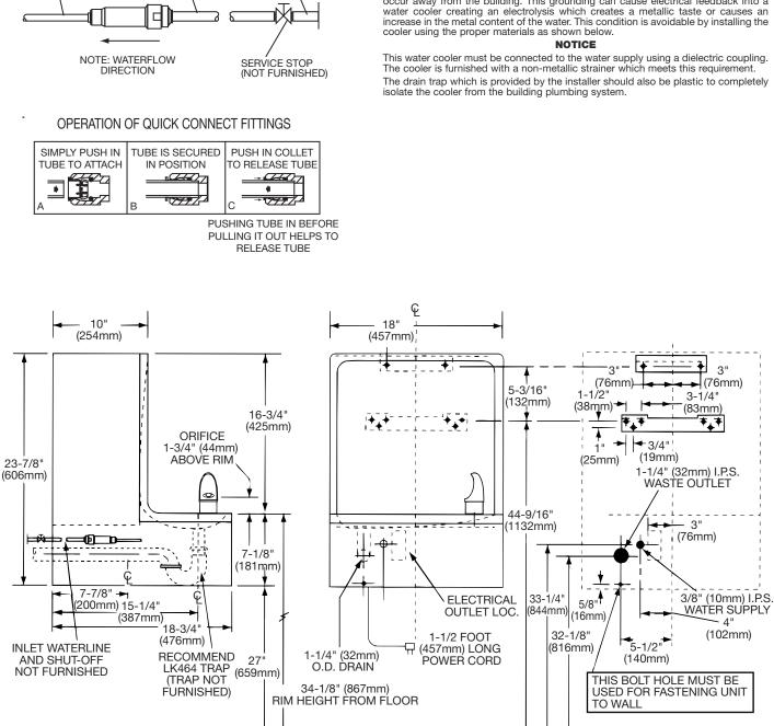
NOTE: INSURE PROPER VENTILATION BY MAINTAINING 6" (152mm) CLEARANCE FROM CABINET LOUVERS TO WALL ON EACH SIDE OF COOLER
