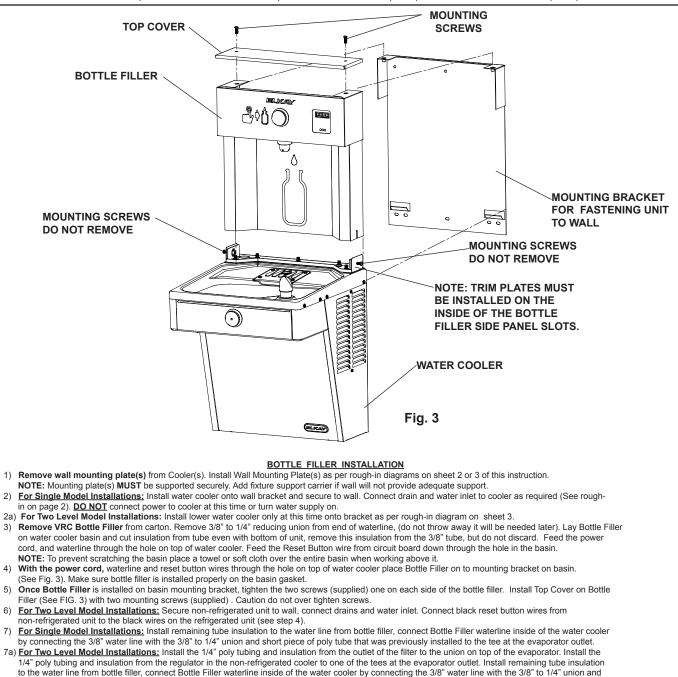
to the water line from bottle filler, connect Bottle Filler waterline inside of the water cooler by connecting the 3/8" water line with the 3/8" to 1/4" union and short piece of poly tube that was previously installed to the tee at the evaporator of the refrigerated cooler.
