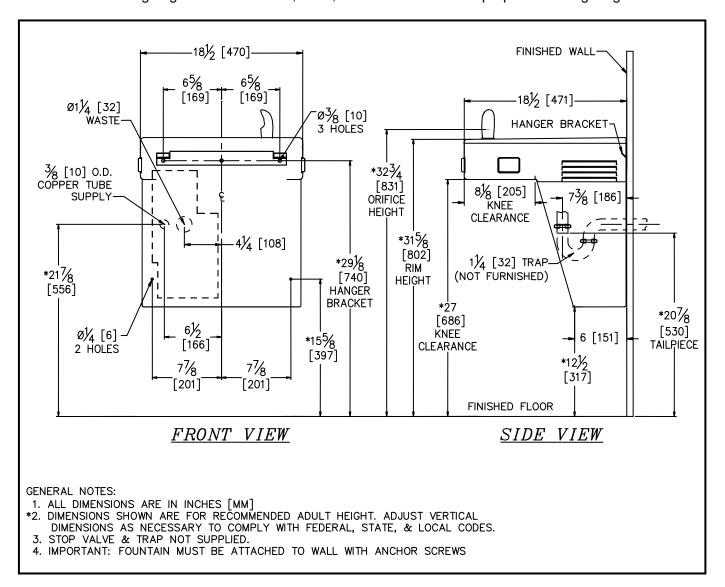
**NOTES:** Dimensions shown for Adult ADA compliant installation. For Child ADA compliant parallel approach installation, decrease height of installation by 3 inches. Provide clear floor space as required. Adjust vertical dimensions as required to comply with federal, state, and local codes.
