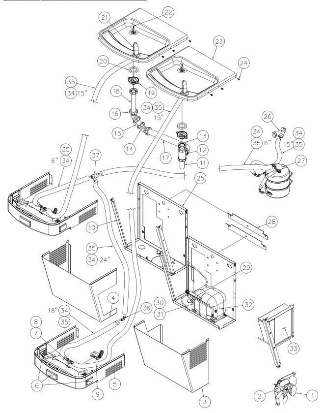
Standard A112108F/B & A112408F/B Refrigerated Bi-Level AquaAccess shown.
